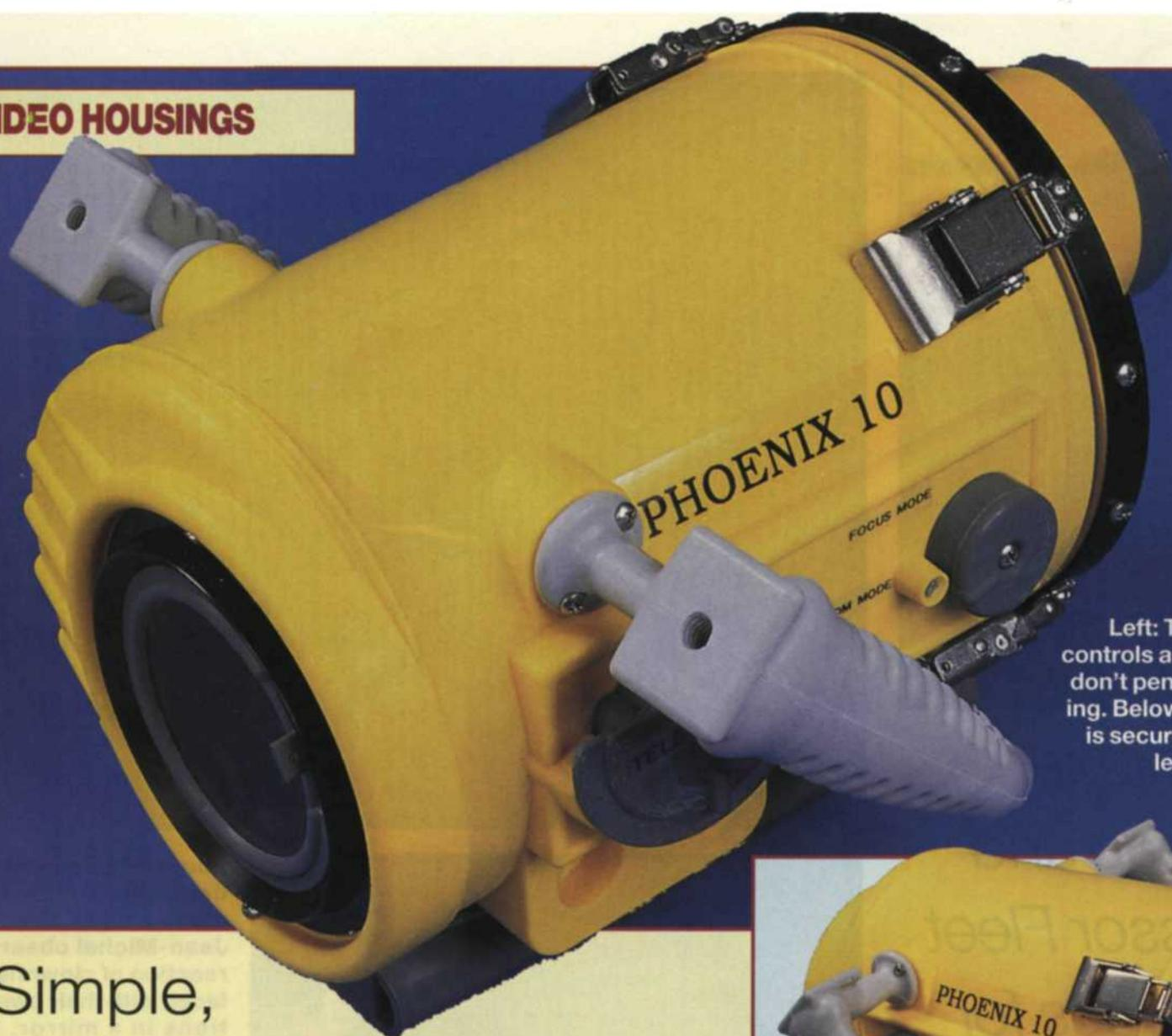
Left: The Phoenix 10's controls are magnetic and don't penetrate the housing. Below: The backplate is secured by four stainless steel clamps.
